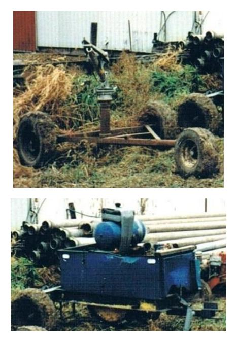
The source of water came from a large rubber hose which trailed behind the "walker" (or sprayer) and was filled by 20-foot-long aluminum pipes. These were laid out to two creek-and-spring-fed
